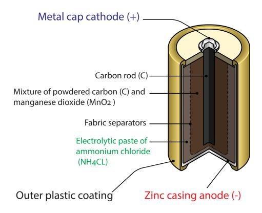
NB Different types of batteries are composed of different chemical combnations. This diagram shows an alkaline battery,
